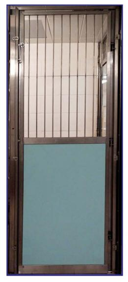
Doors are provided complete with frames, hinges and safety release latch as standard. The standard size is 780mm wide by 2000mm high, however any size can be specified to suit individual requirements.
